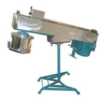
It's a extruder class machine used to extrude the dough into various namkeen components using appropriate dies.
