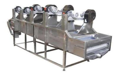
It's a simple machine designed to dry the given product within specified range, by removing extra oil by utilizing appropriate mechanisms; the simplest class of this machine utilize a perforated drum and motor arrangement, to simply centrifuge the excess oil, while continuous line utilize vibrating tray or air dryer type arrangements.
