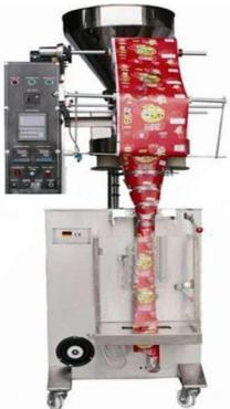
The functioning of machine is simple, it forms an open pouch by two step sealing, followed by filling of chips, nitrogen flushing and final sealing to obtain the namkeen filled packet.
